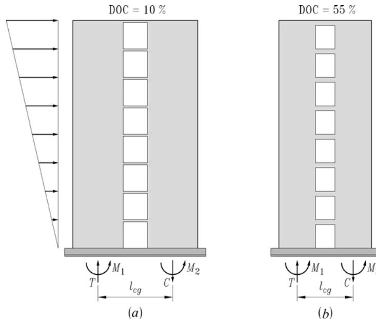
Figure 1. Geometry of wall systems (a) weakly coupled, (b) moderately coupled.
