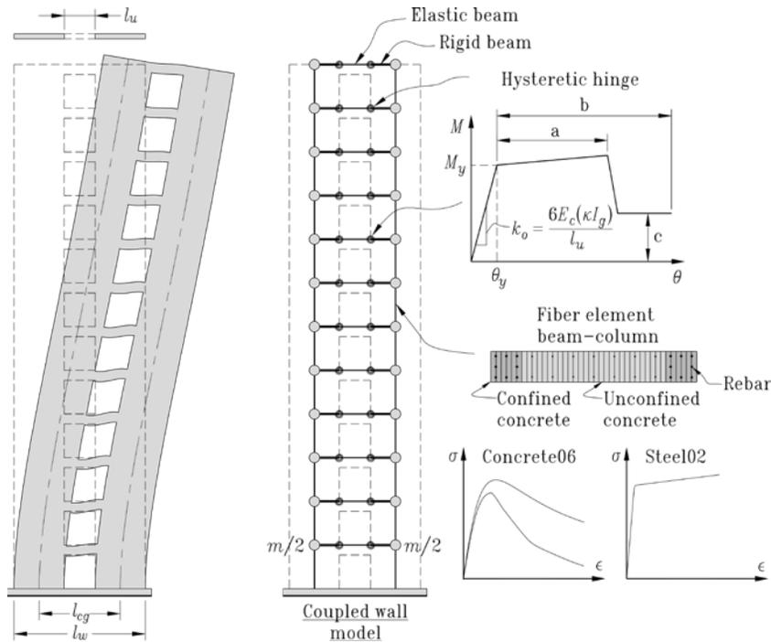
Figure 2. Multilayer beam-column elements on OpenSEES.
